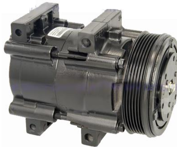
Compressor without Crankcase – No Oil Plug
