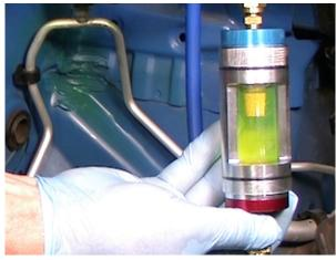
This system has dye already present and can be directly checked with a UV leak detector without adding additional dye.
