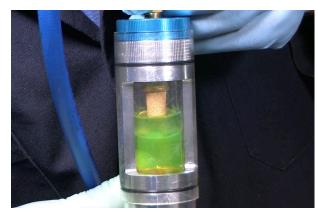
The refrigerant and oil have separated in this system which could lead to compressor failure. This system also has dye already present so more would be unnecessary.
